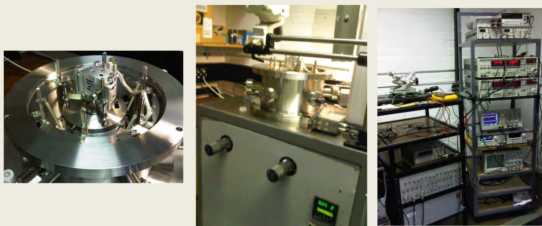
Figure 6: Vacuum multimode SPM; NT-MDT microscope with magnetic damping, and electronics for detection of DC and AC thermal signals, UFM.
